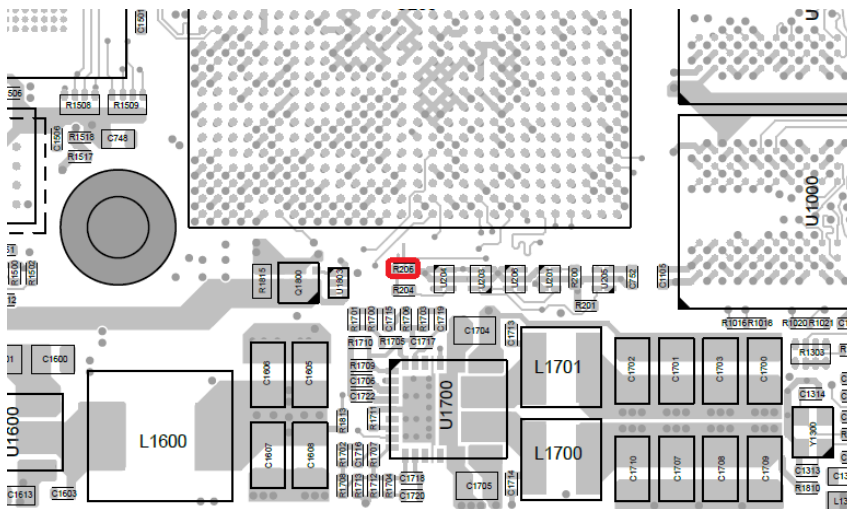
Figure 14: JTAG Boot Mode Resistor - Assembly Drawing Top View (lower center part)
